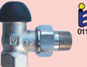
011 | <b>HERZ-TS-90 H thermostatic valve<br/>Angle model</b><br>Radiator connection with cone.<br>Universal models with special socket for threaded pipe and compression adapter connection.<br>DIN dimensions.         | 1/2  | 1 7724 26    | 20        |   |
